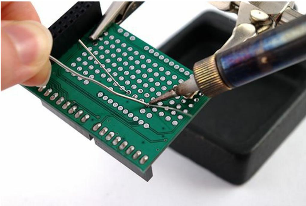
4. As the solder flows, you'll see it drawn down into the hole in the board. This is an indication that the area is hot enough for a good solder joint. If the solder floats, it indicates that the area is not yet hot enough.
