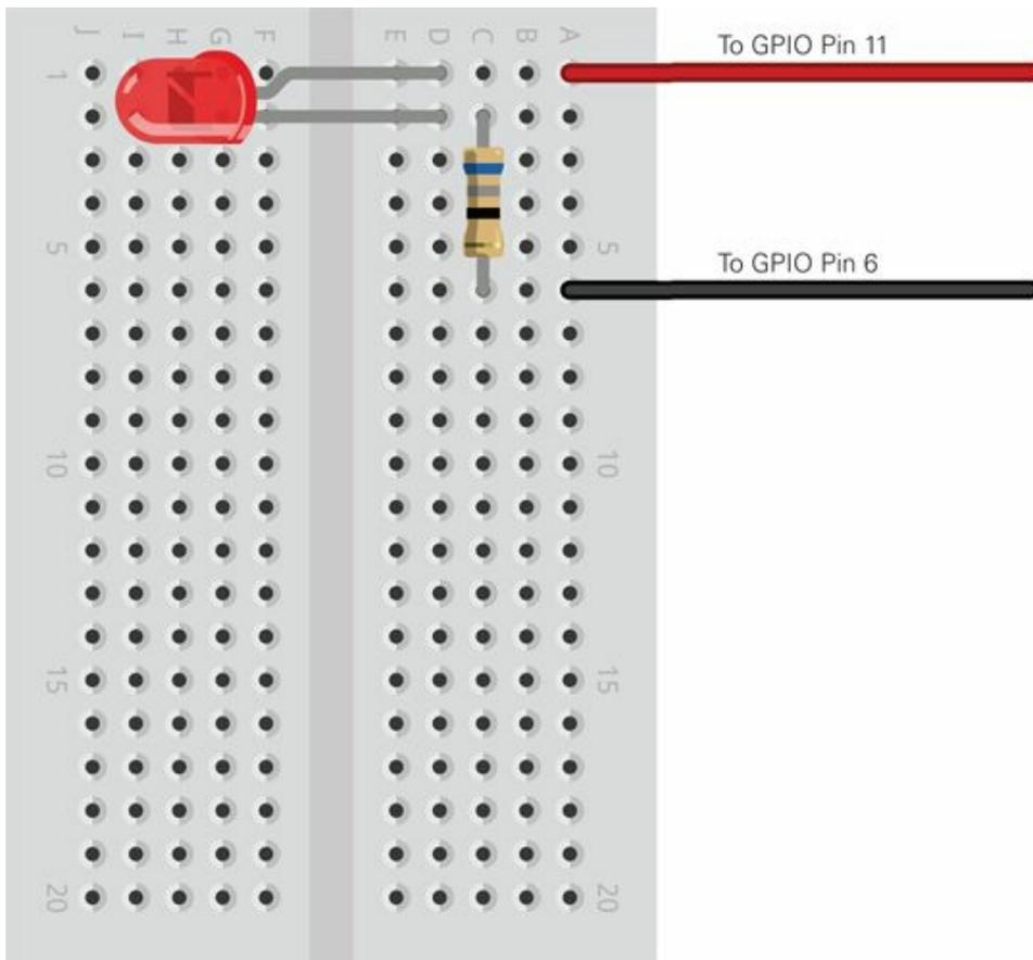
At this point, nothing will happen. That's perfectly normal: by default, the Raspberry Pi's GPIO pins are switched off. If you want to check your circuit immediately, move the wire from Pin 11 to Pin 1 to make the LED light up. Be careful not to connect it to Pin 2, though: a current-limiting resistor suitable for a 3.3 V power supply will be inadequate to protect the LED when connected to 5 V. Remember to move the wire back to Pin 11 before continuing.
