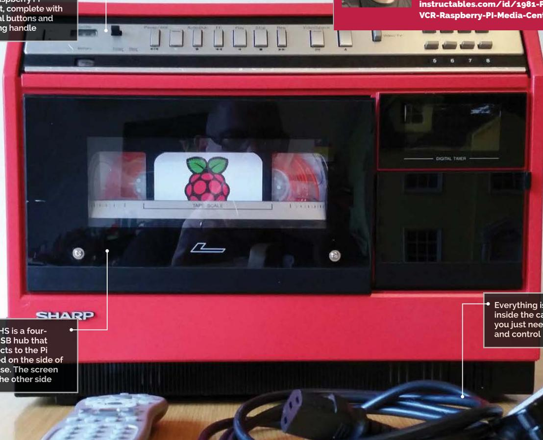
The VHS is a four-port USB hub that connects to the Pi located on the side of the case. The screen is on the other side
