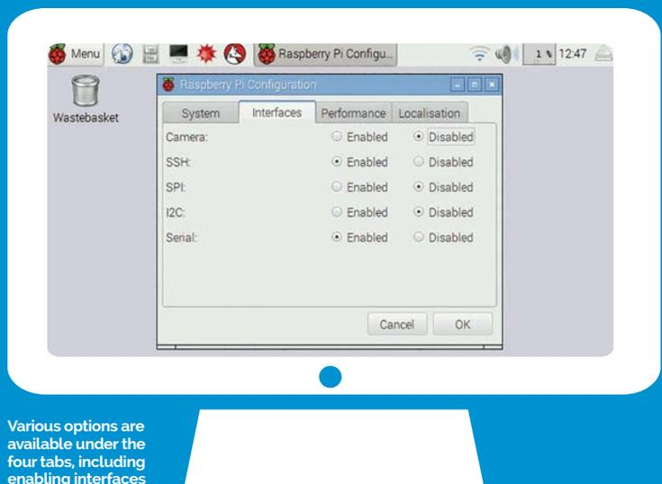
Various options are available under the four tabs, including enabling interfaces
