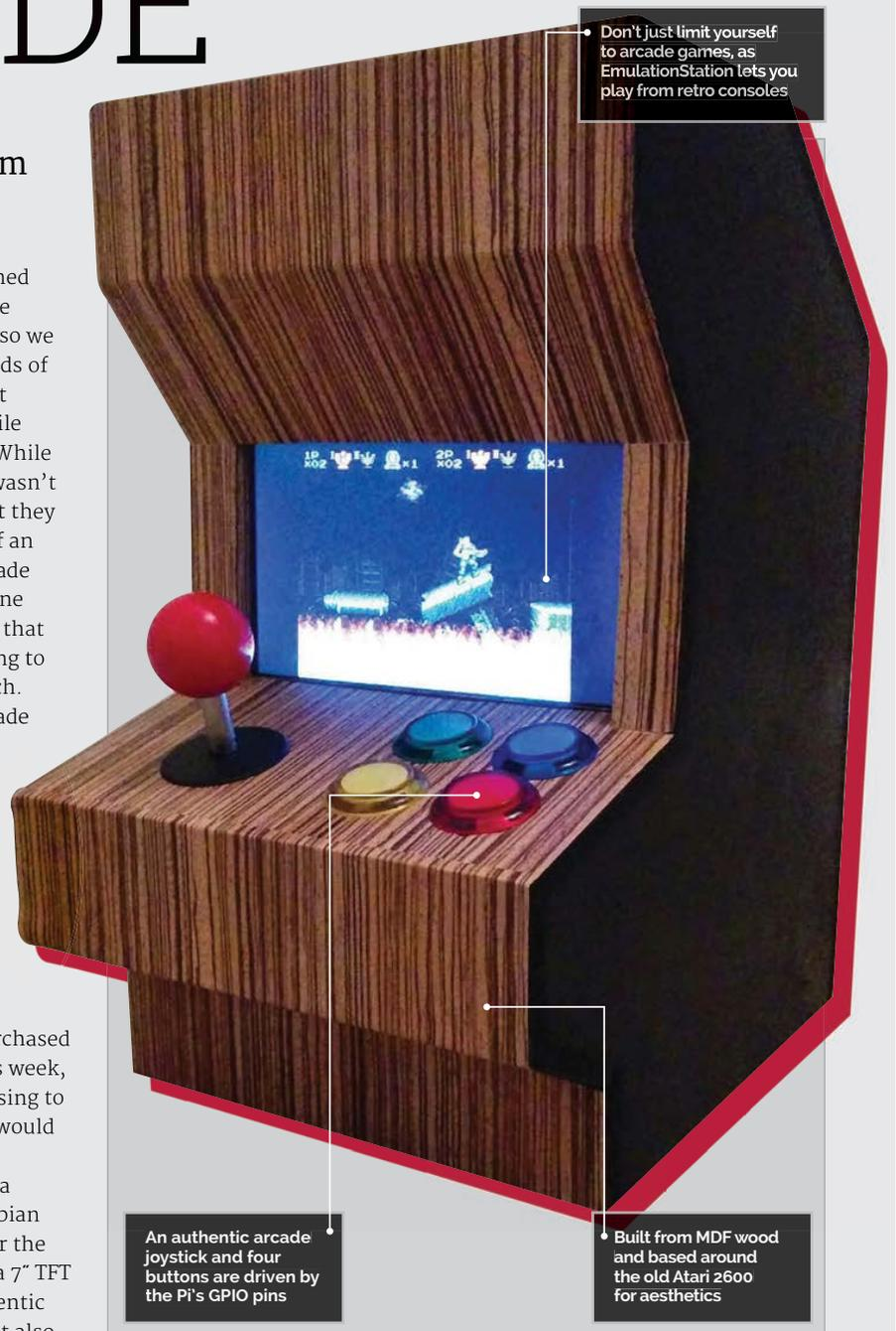
An authentic arcade joystick and four buttons are driven by the Pi's GPIO pins
