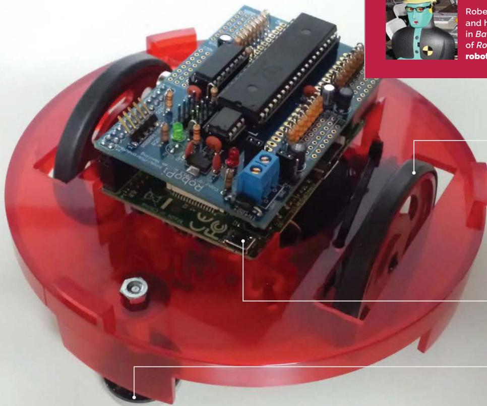
Rectangles are cut into the base, and servos with wheels are glued beneath
