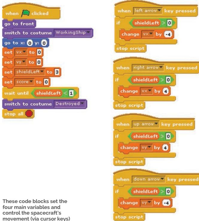
These code blocks set the four main variables and control the spacecraft's movement (via cursor keys)
