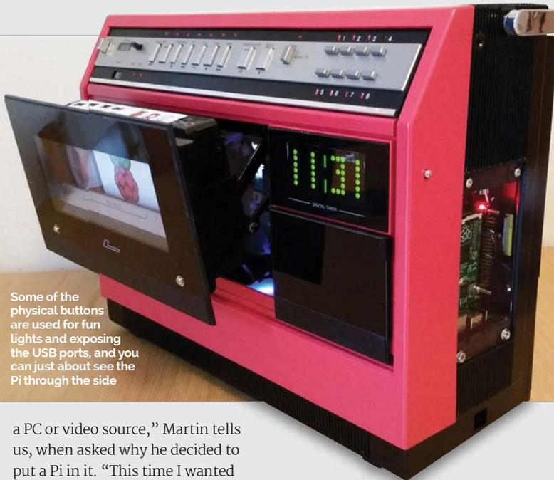
Some of the physical buttons are used for fun lights and exposing the USB ports, and you can just about see the Pi through the side
