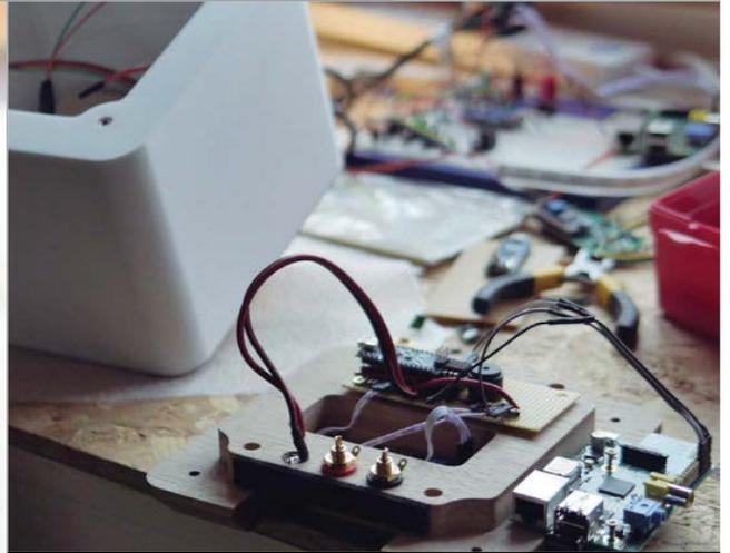
**Above** The project also uses an Arduino Nano, partly to help reduce the CPU load on the Raspberry Pi, which uses up to 70% on decrypting Spotify tracks
