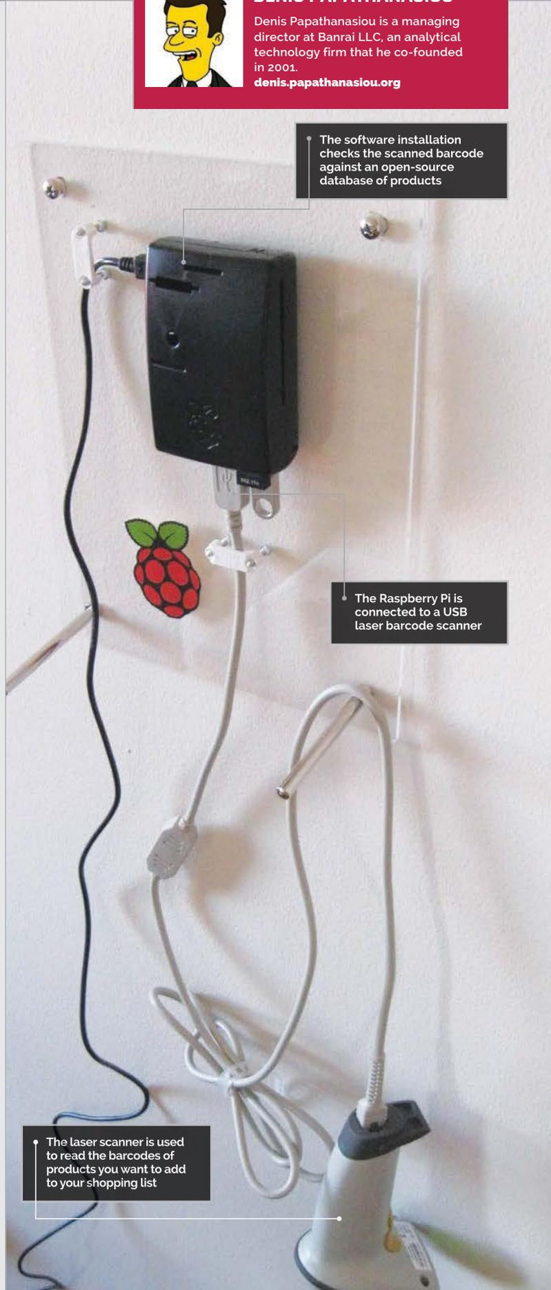
The software installation checks the scanned barcode against an open-source database of products
