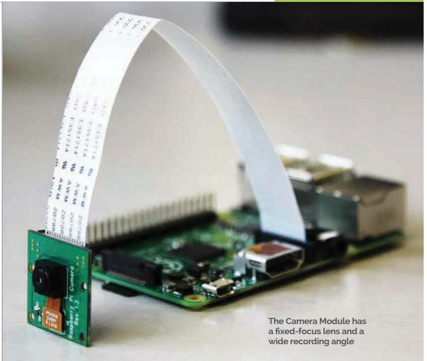
The Camera Module has a fixed-focus lens and a wide recording angle
