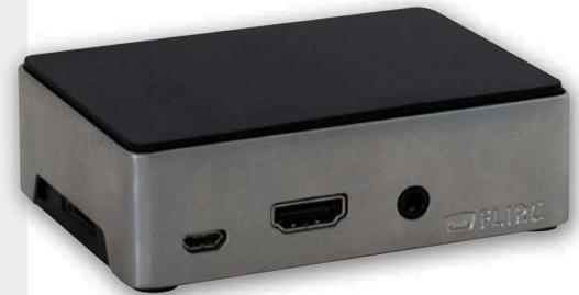
The Flirc Case has a very solid construction as it's made from a solid aluminium shell with a matte, rubberised plastic top and base. The aluminium finish gives the case a premium feel, too, which is always a bonus. Unlike the other cases on test, it comes with a built-in heatsink. It's easy to put together, using four screws to secure it.
