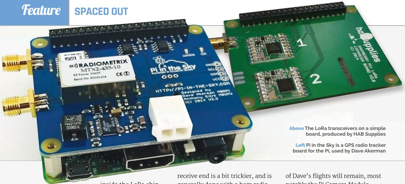
**Above** The LoRa transceivers on a simple board, produced by HAB Supplies
