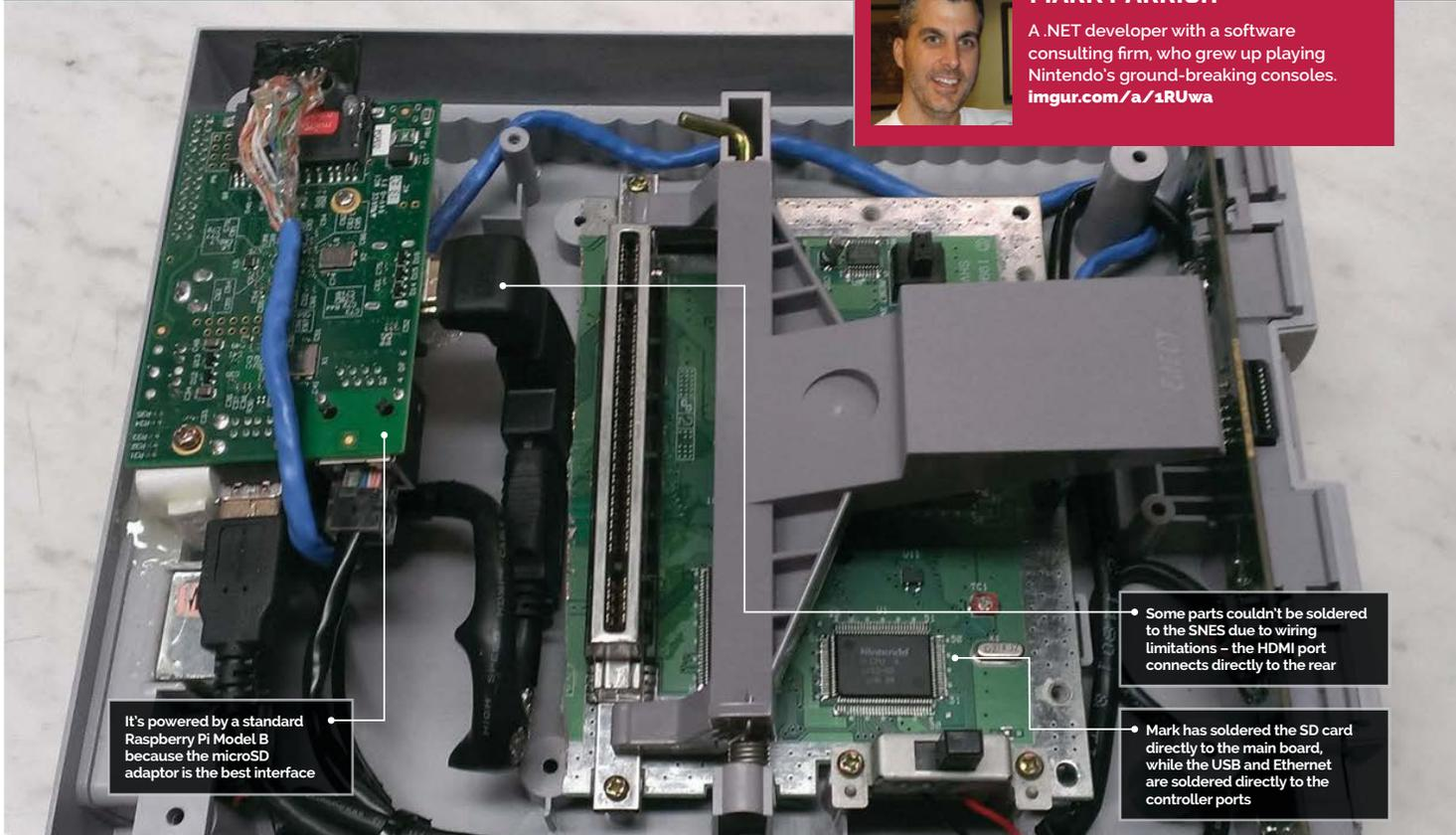
It's powered by a standard Raspberry Pi Model B because the microSD adaptor is the best interface
