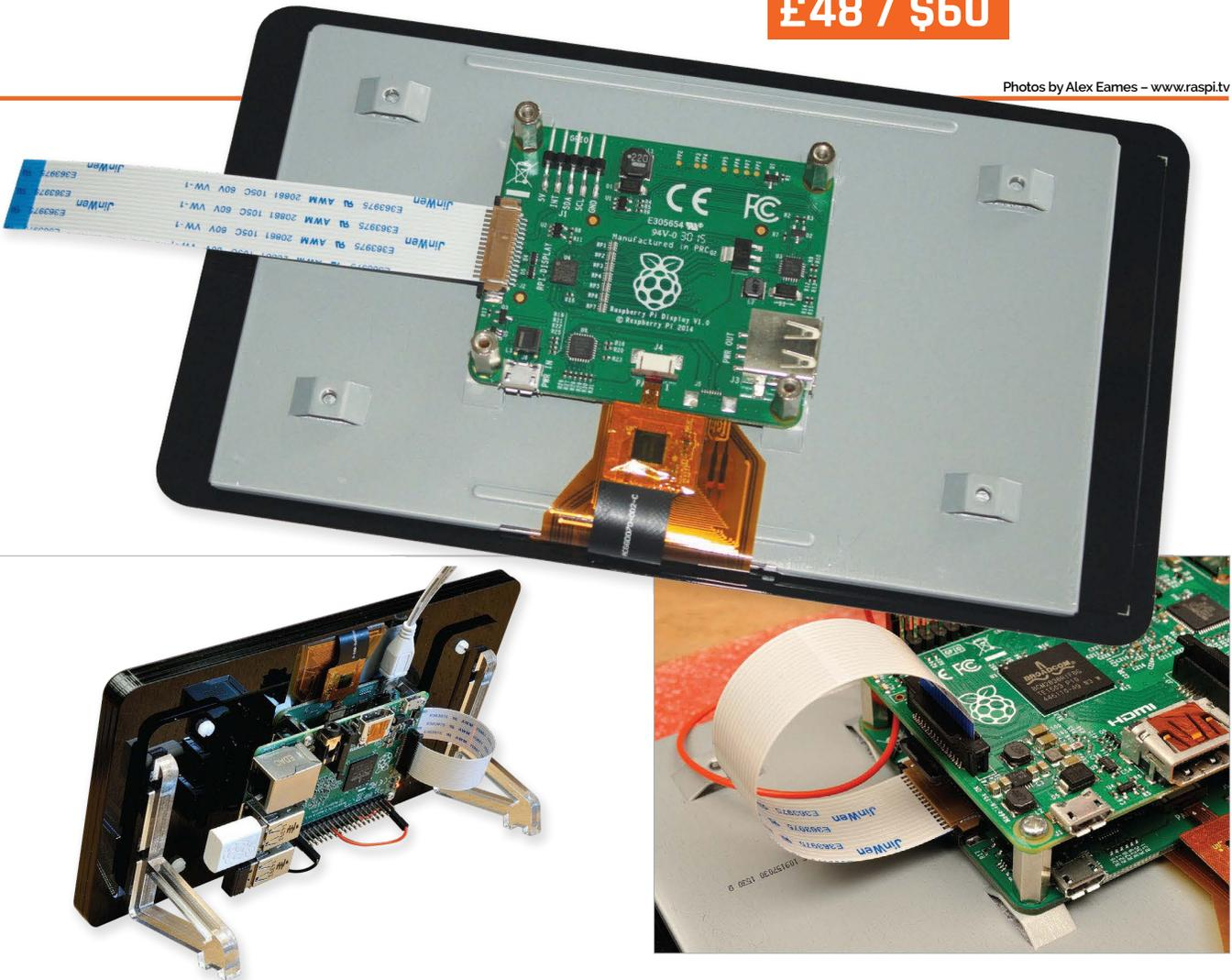
screws you need to safely secure it to your Pi, a DSI ribbon cable, and four jumper wires for both power and communications. Pimoroni has also produced an excellent Pi-bow-esque bezel with integrated stand in different colours. For a small premium, you can add your chosen colour to the shopping basket so you don't have to worry about propping the screen up or 3D-printing your own solution.
