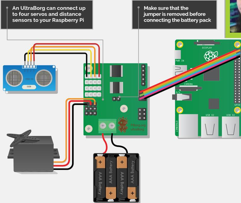
**Below** The various parts connected to UltraBorg, just missing the Raspberry Pi. The sensor is attached to one of PiBorg's optional mounting kits
