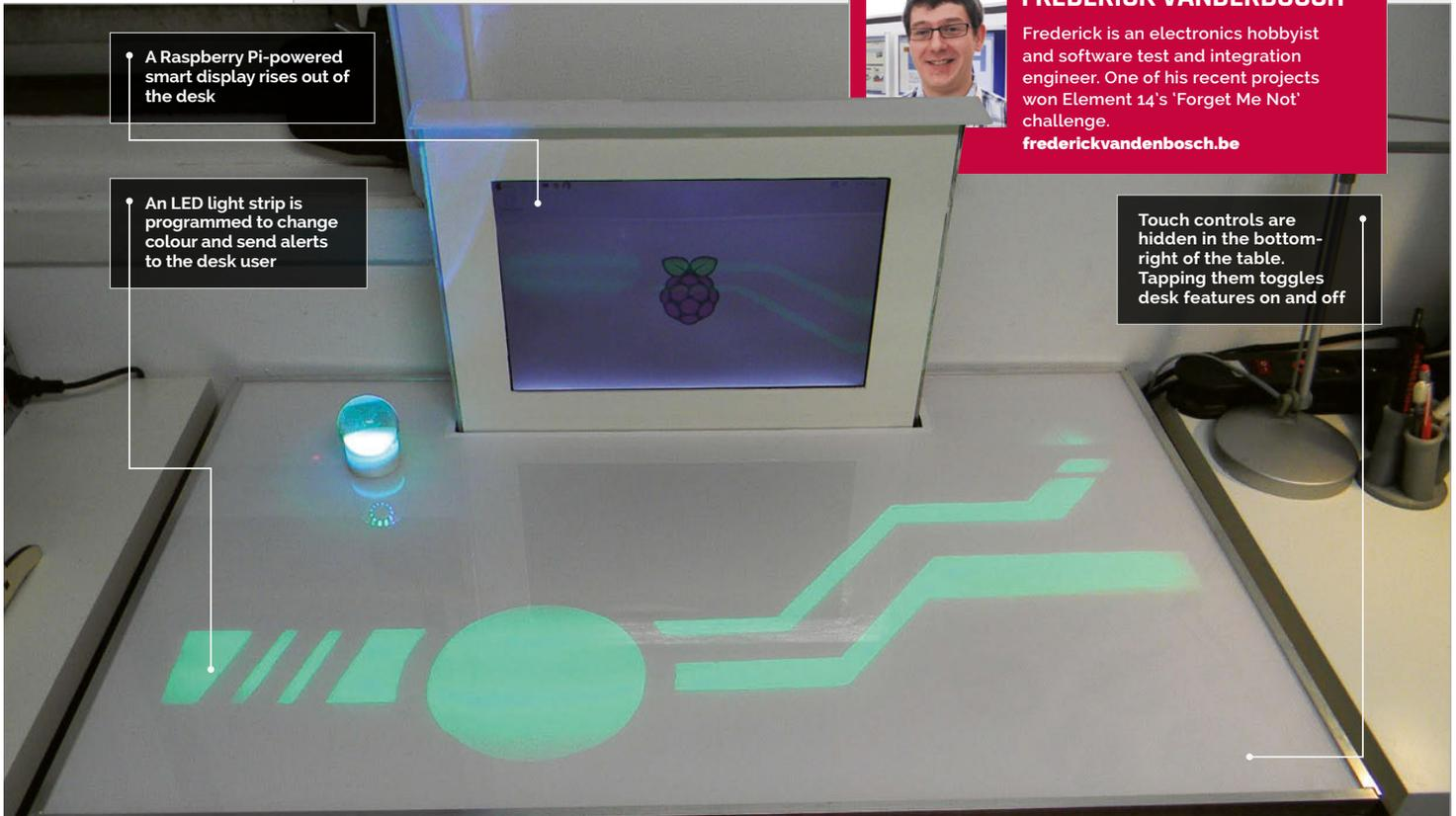
A Raspberry Pi-powered smart display rises out of the desk
