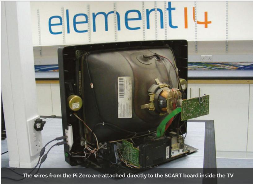
The wires from the Pi Zero are attached directly to the SCART board inside the TV
