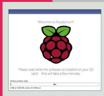
NOOBS automatically copies all the files needed to run Raspbian onto your SD card
