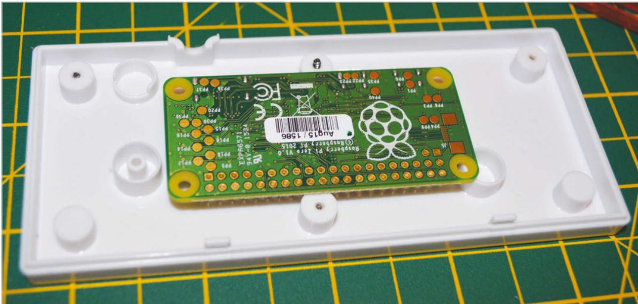
We used a Sharpie to mark out the cuts we needed to make by periodically laying the Zero over the backplate as we worked
