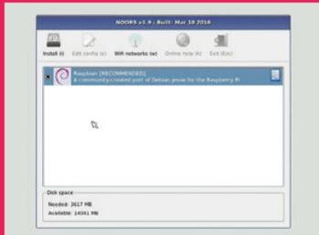
With the NOOBS files copied across, remove the micro SD card from your computer and slot it into your Raspberry Pi. Now connect the keyboard, mouse, and HDMI cable. Finally, attach the USB power to boot up the Raspberry Pi.
